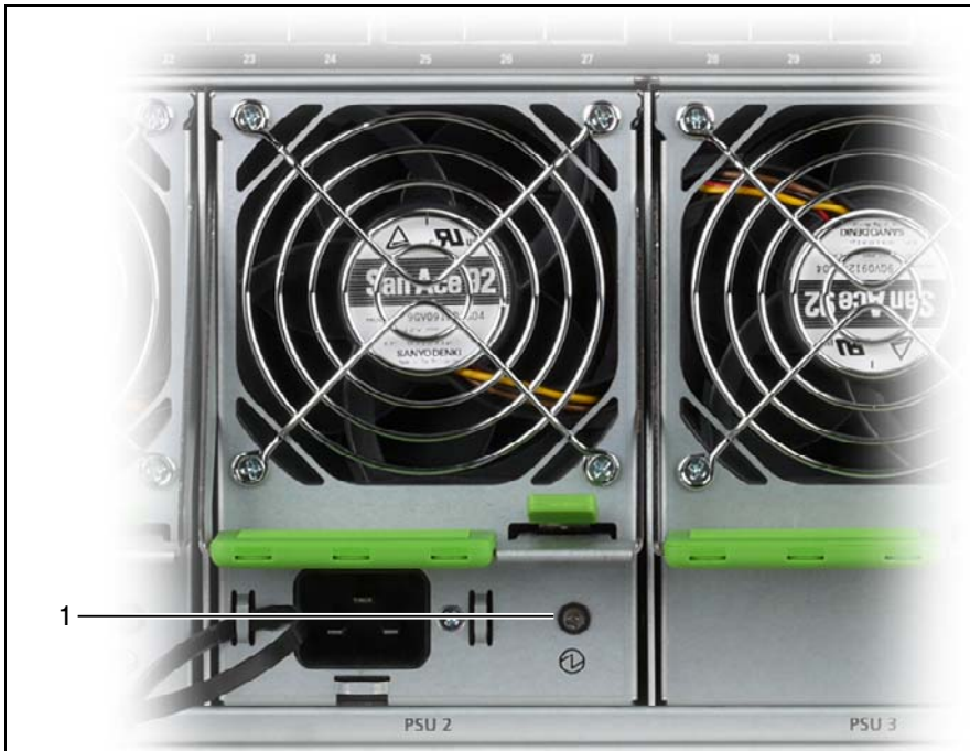
Figure 17: Indicator on the hot-plug power supply unit
